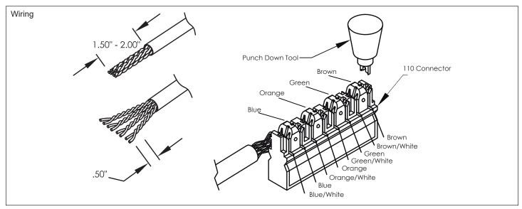
Terminate as indicated. Follow the color-code and only use 110 punch-down tool to terminate the wires. TIA-570 residential wiring standard specifies TIA-568-A color code wiring as the standard for residential installations.
