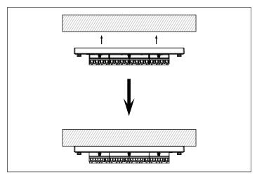
Find a flat, clean surface and press firmly on the module to adhere to the desired surface.
