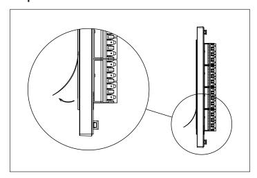
Peel off film backing from each of the self-adhesive.
