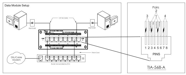
This module supports data connections for 8 locations. Connect one end of a patch cord to a jack and the other end to the router after identifying the port you want to activate.
